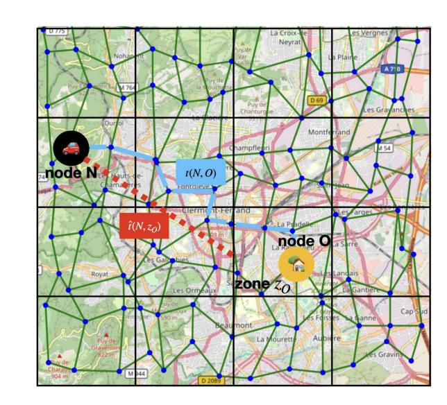
Illustration of the partition of the road network and a basic example. An SAV is scheduled to pass the node N during a certain time window. To know departing from N, whether it can reach the origin O of the target request, we first check if it can approximately pass the zone Zo using the estimated node-zone travel time (represented by the red dotted line).
