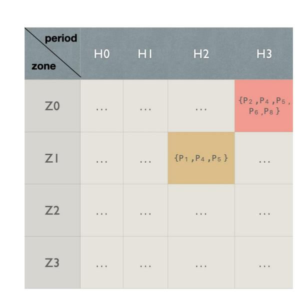
The fleet filter M<sup>v</sup><sub>aux</sub> for the candidate vehicle v. The new query's origin is related to the zone Z1 and the period H2, while its destination is related to the zone Z0 and the period H3. The corresponding cells M<sup>v</sup><sub>aux</sub>[Z1, H2] and M<sup>v</sup><sub>aux</sub>[Z0, H3] are thus respectively taken into account while
