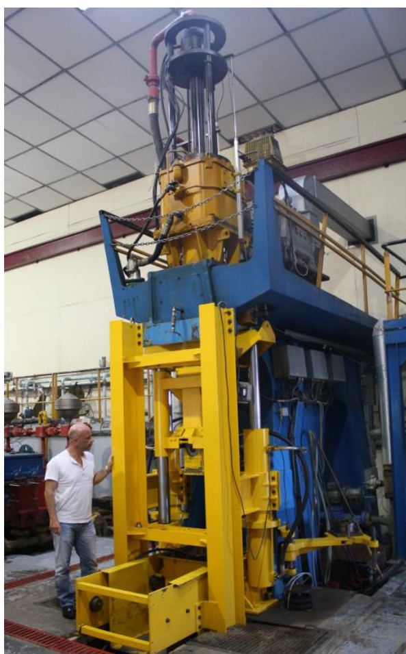
Banc de forage MINES ParisTech
